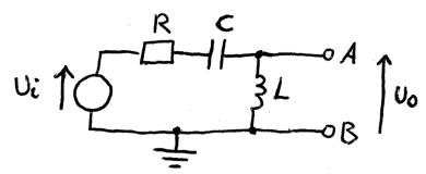
Consider the circuit above. The reactances at some specific frequency are  $X_C = 40 \Omega$ ,  $X_L = 90 \Omega$  and take for the resistor  $R = 50 \Omega$ . The voltage source delivers a current of magnitude  $|i_{in}| = 0.1 A$ .
